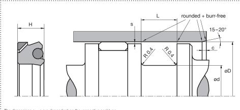
The dimensions s + c are dependent on the respective seal type.
